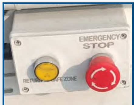
Emergency Stop in Bucket
